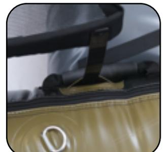
Note: The LCS Stripping apron is designed to come out of stay pockets incase the boat becomes capsized.
